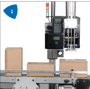
1 Labelling in motion, different sized products up to 30 labels per minute.
